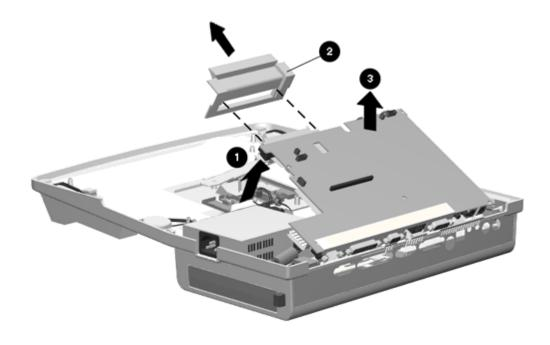
Figure 6-18. Removing the Main Board Assembly
